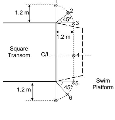
NB. Microphones shall be located as close to 1.2m from the hull as practically possible. Similarly they shall be located as close to 1.2m from the water surface as practically possible.
